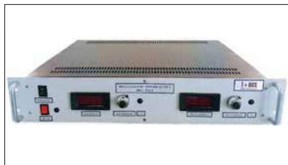
Indigenously developed Switch Mode Power Supply (SMPS) for high voltage DC power
