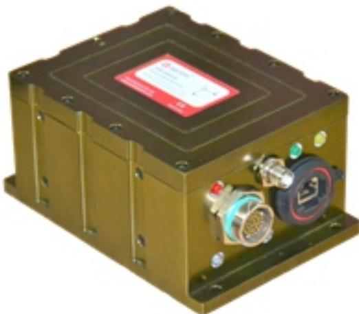
**P.2.3.2.6 Inertial Navigation system with GPS for UAV application & other defense applications**
